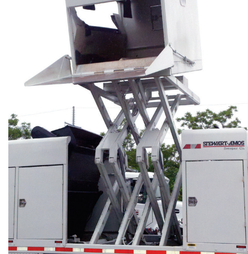
Massive quad (4) "X" style lift scissors with four corner lift provide exceptional hopper stability especially when dumping wet, unbalanced or sticky debris.
