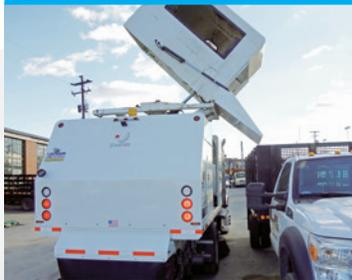
Variable dump height hopper (up to 12' high) with 44" extra-long dump door easily reaches most dump trucks.
