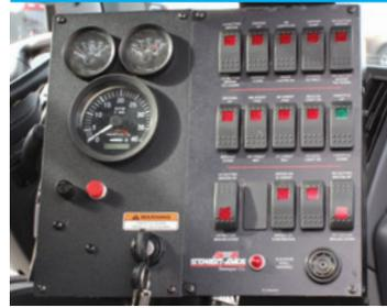
Vertically-mounted control panel is 6-way adjustable for easy & ergonomic viewing. One-touch sweeping allows for operator to preset functions. Brooms raise automatically in reverse.
