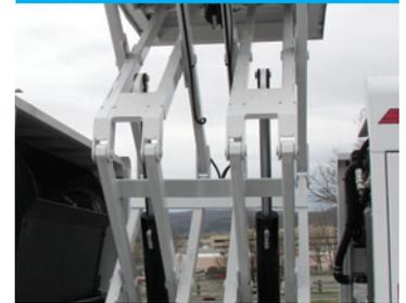
Massive double "X" style lift scissors & 4-corner hopper lift ensure exceptional hopper stability when dumping wet, unbalanced, or sticky debris.
