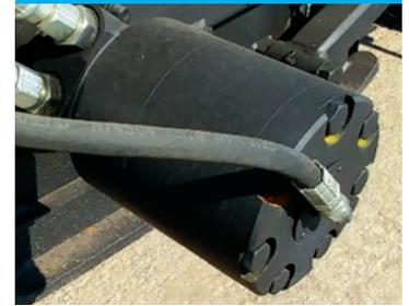
Case drains for all the hydraulic motors protect shaft seals from pressure leaks, minimizing repairs & replacements.
