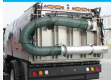
Optional 10' Auxiliary Suction Hose with 4' aluminum tube helps clean storm drains.
