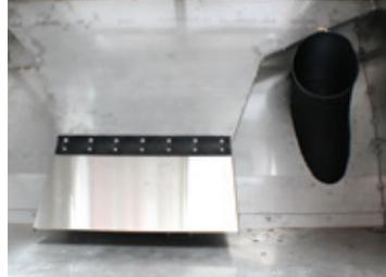
Stainless steel, centrifugal dust separator located inside the hopper separates fines from the air stream.
