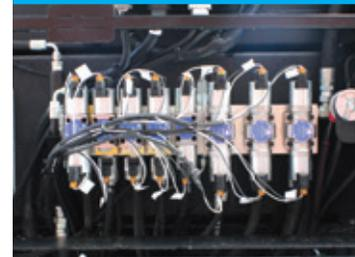
Effectively simple electric-over hydraulic valve system has reliable & easy-to-replace components. Onboard pressure gauge allows for simple servicing.
