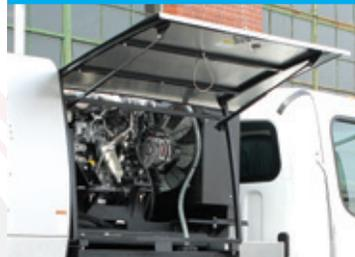
Stainless steel engine shrouds are compact, protective & noise reducing. Gull wing design makes it easier and faster to service power plant without raising an interconnected hopper/shroud assembly.
