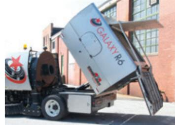
The top-mounted hopper cover opens automatically during dumping cycle to provide quicker, easier & safer cleaning of stainless steel screens & hopper.
