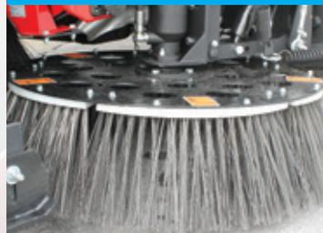
Spring-balanced, free-floating gutter brooms automatically apply correct surface pressure for maximum broom wear life. In-cab gutter broom electric tilt is standard.
