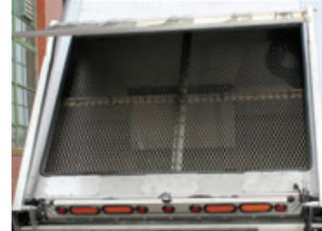
28 ft<sup>2</sup> stainless steel debris separator screens maximize sweeping productivity. Screens can be easily cleaned from outside of unit. Bolt-in design makes screen replacement easy.
