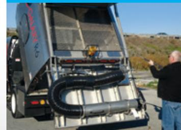
Optional High-Pressure Wash Down System with 50' hose reel & spray wand allow separator screens & hopper to be cleaned at any time which can improve vacuum performance.
