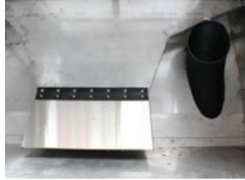
Stainless steel, centrifugal dust separator located inside the hopper separates fines from the air stream.
