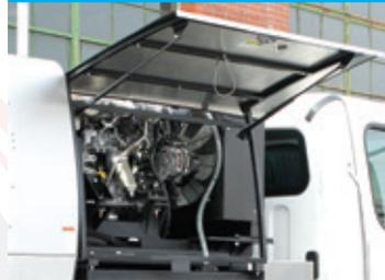
Stainless steel engine shrouds are compact, protective & noise reducing. Gull wing design makes it easier & faster to service power plant without raising an interconnected hopper/shroud assembly.
