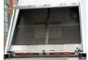
28 ft² stainless steel debris separator screens maximize sweeping productivity. Screens can be easily cleaned from outside of unit. Bolt-in design makes screen replacement easy.
