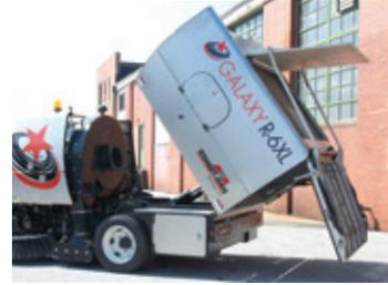
The top-mounted hopper cover opens automatically during dump cycles to provide quicker, easier & safer cleaning of stainless steel screens & hopper.
