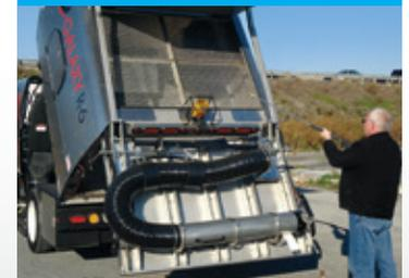
Optional High-Pressure Wash Down System with 50' hose reel & spray wand allow separator screens & hopper to be cleaned at any time which can improve vacuum performance.
