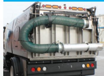
Optional rear-mounted 10' Auxiliary Suction Hose with 4" aluminum tube helps clean storm drains.
