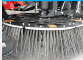
Spring-balanced, free-floating gutter brooms automatically apply correct surface pressure for maximum broom wear life. In-cab gutter broom electric tilt is standard.
