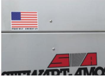
Bolt-together, stainless steel hopper panels (no welds) are easier & more economical to replace if damaged. Hopper comes with a 5-year "no rust-through" factory warranty.
