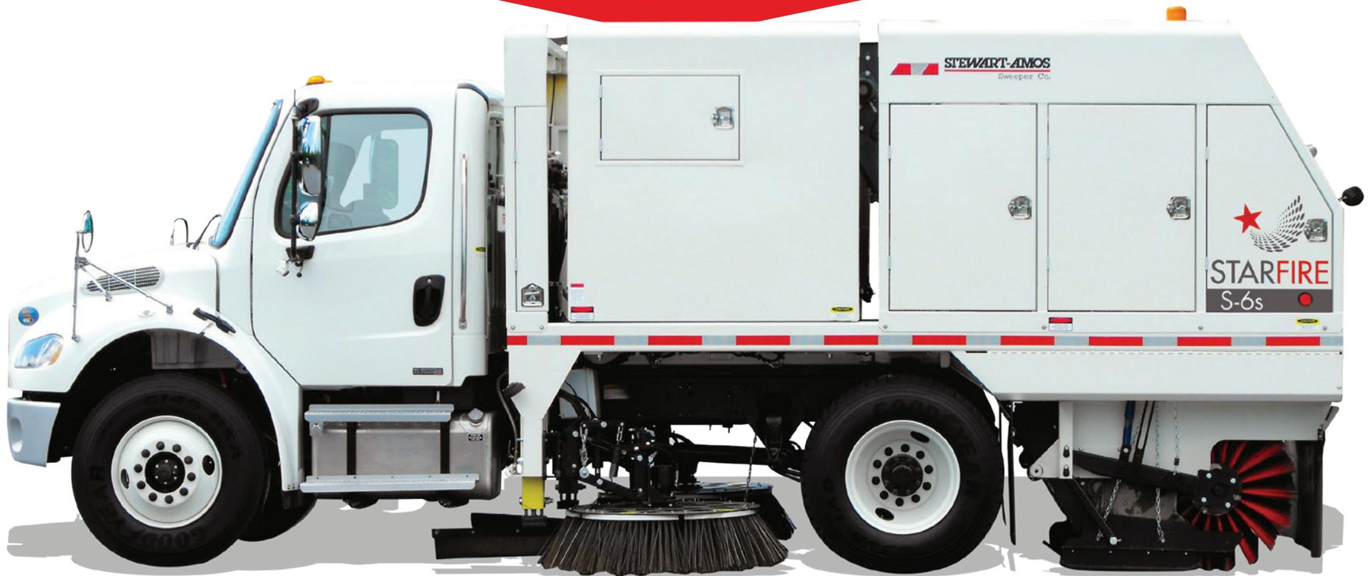
*An Effectively Simple, Single Engine, 6 yd<sup>3</sup> Broom Sweeper Mounted on a Full-Size Commercial Chassis.*
