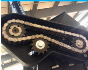
Off-set hydraulic elevator drive motor is protected against shock loading.
