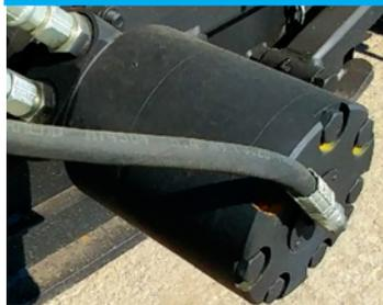
Case drains for all the hydraulic motors protect shaft seals from pressure leaks minimizing repairs & replacements.
