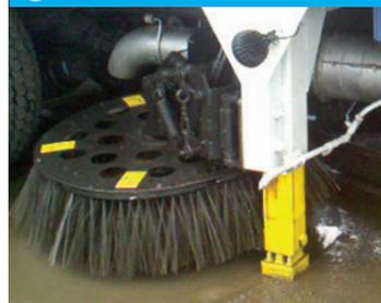
To maximize safety, front stabilizers automatically deploy during hopper dumping. This provides added stability when dumping heavy, sticky, or unbalanced loads.
