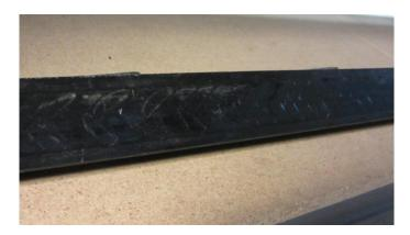
The shoes could get bent when turning a corner and the shoe getting hung up in a crack or on a manhole. During milling operations they can get bent going into or out of a mill cut. If the shoes get bent they will not seal against the main broom and could leave a trail. There is an optional drag brush arrangement that can be bolted onto the main broom arm and the drag shoes are removed. The drag brush option can leave trails on regular street sweeping.
