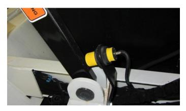
When a proximity switch is activated a small LED light on the back of the switch lights. When the steel is out of proximity to the switch it breaks contact and LED goes out.
