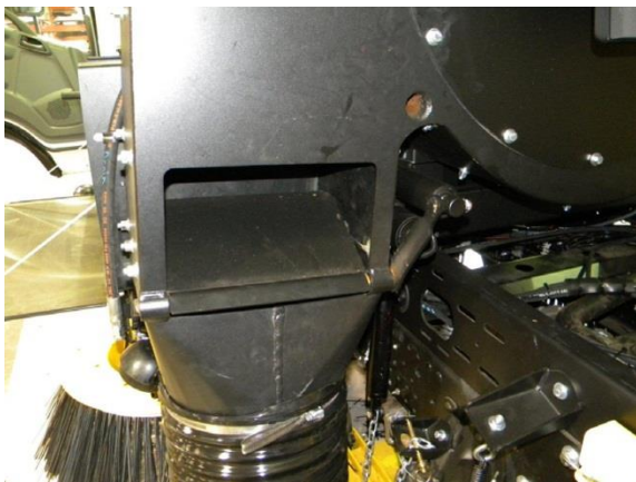
Air bleeder door shown 100% closed
