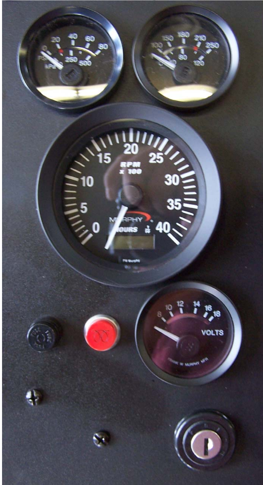
Figure 2: Engine Control Box
