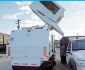
Variable dump height hopper (up to 12' high) with 44" extra-long dump door easily reaches most dump trucks.
