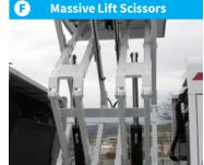
Massive double "X" style lift scissors & 4-corner hopper lift ensure exceptional hopper stability when dumping wet, unbalanced, or sticky debris.
