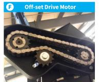
Off-set hydraulic elevator drive motor is protected against impacts.
