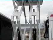
Massive double "X" style lift scissors & 4-corner hopper lift ensure exceptional hopper stability when dumping wet, unbalanced, or sticky debris.
