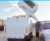
Variable dump height hopper (up to 11' high) with 44" extra-long dump door easily reaches most dump trucks.
