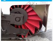
Main broom channeler (optional) effectively sweeps large quantities or bulky & light debris (leaves/pine straw). Self-adjusting as main broom wears.
