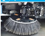
Spring-balanced, free-floating main & gutter brooms automatically apply correct surface pressure for maximum broom wear life. In-cab gutter broom electric tilt is standard.
