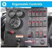
Vertically-mounted control panel is 6-way adjustable for easy & ergonomic viewing. One-touch sweeping allows operator to preset functions. Brooms raise automatically in reverse.
