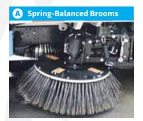
Spring-balanced, free-floating main & gutter brooms automatically apply correct surface pressure for maximum broom wear life. In-cab gutter broom electric tilt is standard.
