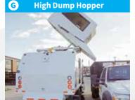
Variable dump height hopper (up to 11' high) with 44" extra-long dump door easily reaches most dump trucks.
