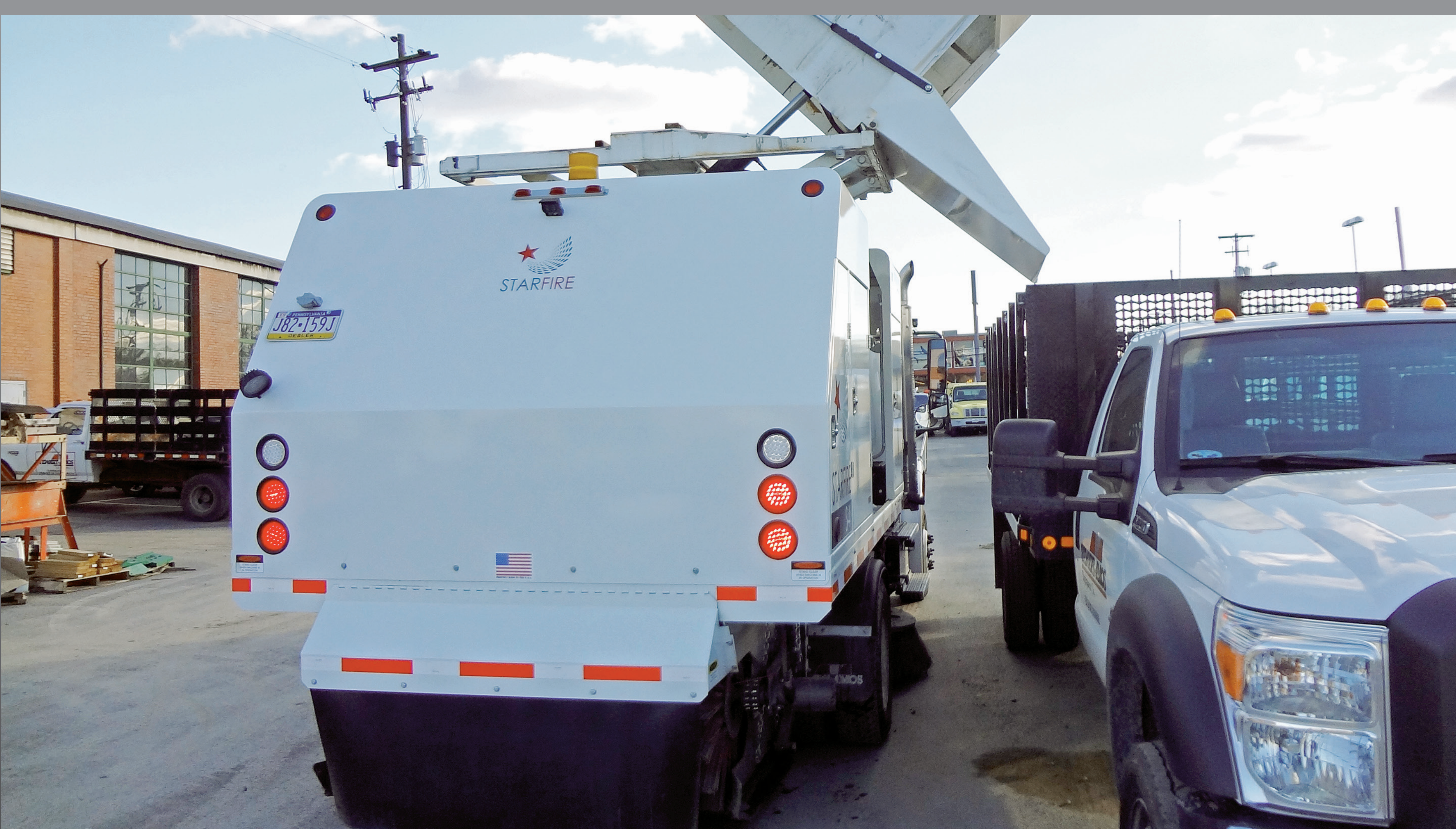
Variable Height Dumping from 16" to 11'
