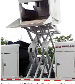
Massive quad (4) "X" style lift scissors with four corner lift provide exceptional hopper stability especially when dumping wet, unbalanced or
