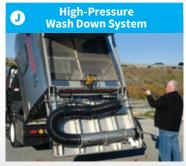
Optional High-Pressure Wash Down System with 50' hose reel & spray wand allow separator screens & hopper to be cleaned at any time which can improve vacuum performance.
