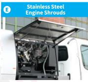
Stainless steel engine shrouds are compact, protective & noise reducing. Gull wing design makes it easier and faster to service power plant without raising an interconnected hopper/shroud assembly.
