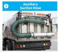
Optional 10' Auxiliary Suction Hose with 4' aluminum tube helps clean storm drains.
