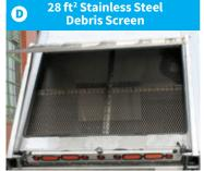
28 ft<sup>2</sup> stainless steel debris separator screens maximize sweeping productivity. Screens can be easily cleaned from outside of unit. Bolt-in design makes screen replacement easy.
