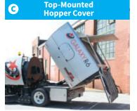
The top-mounted hopper cover opens automatically during dumping cycle to provide quicker, easier & safer cleaning of stainless steel screens & hopper.
