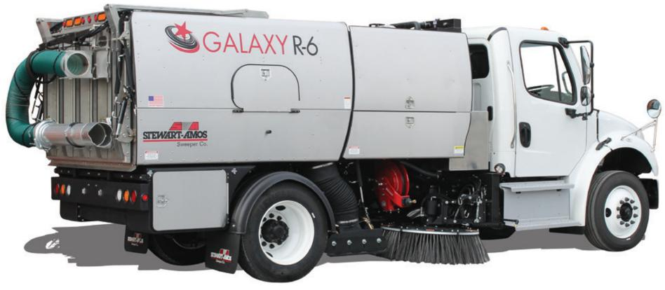
An *Effectively Simple*, Full-Featured 6 yd<sup>3</sup> Regenerative Air Street Sweeper Mounted on a Mid-Sized, Non-CDL Chassis
