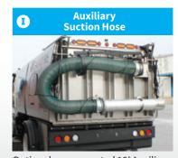
Optional rear-mounted 10' Auxiliary Suction Hose with 4' aluminum tube helps clean storm drains.
