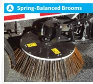
Spring-balanced, free-floating main & gutter brooms automatically apply correct surface pressure for maximum broom wear life. In-cab gutter broom electric tilt is standard.
