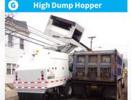
Variable dump height hopper (up to 12' 2" high) with 54" extra-long dump door easily reaches most dump trucks.
