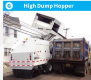
Variable dump height hopper (up to 12' 2" high) with 54" extra-long dump door easily reaches most dump trucks.
