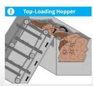
An extended 12-flight elevator maximizes hopper loading by filling from the top down instead of from the side. This reduces unused hopper space to increase productivity.
